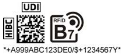
Fig. 4) UDI applied on a product with Data Matrix and RFID
