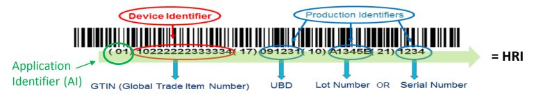
The Human Readable Interpretation (HRI) below the bar code is **used for the human eye to determine the information encoded in the bar code** without need to scan the barcode. The **Als are data delimiters** and are **not** part of the data set. Therefore, the **Als should not be displayed in forms, electronic data interchange (EDI), electronic systems and databases as part of the data-set.**
